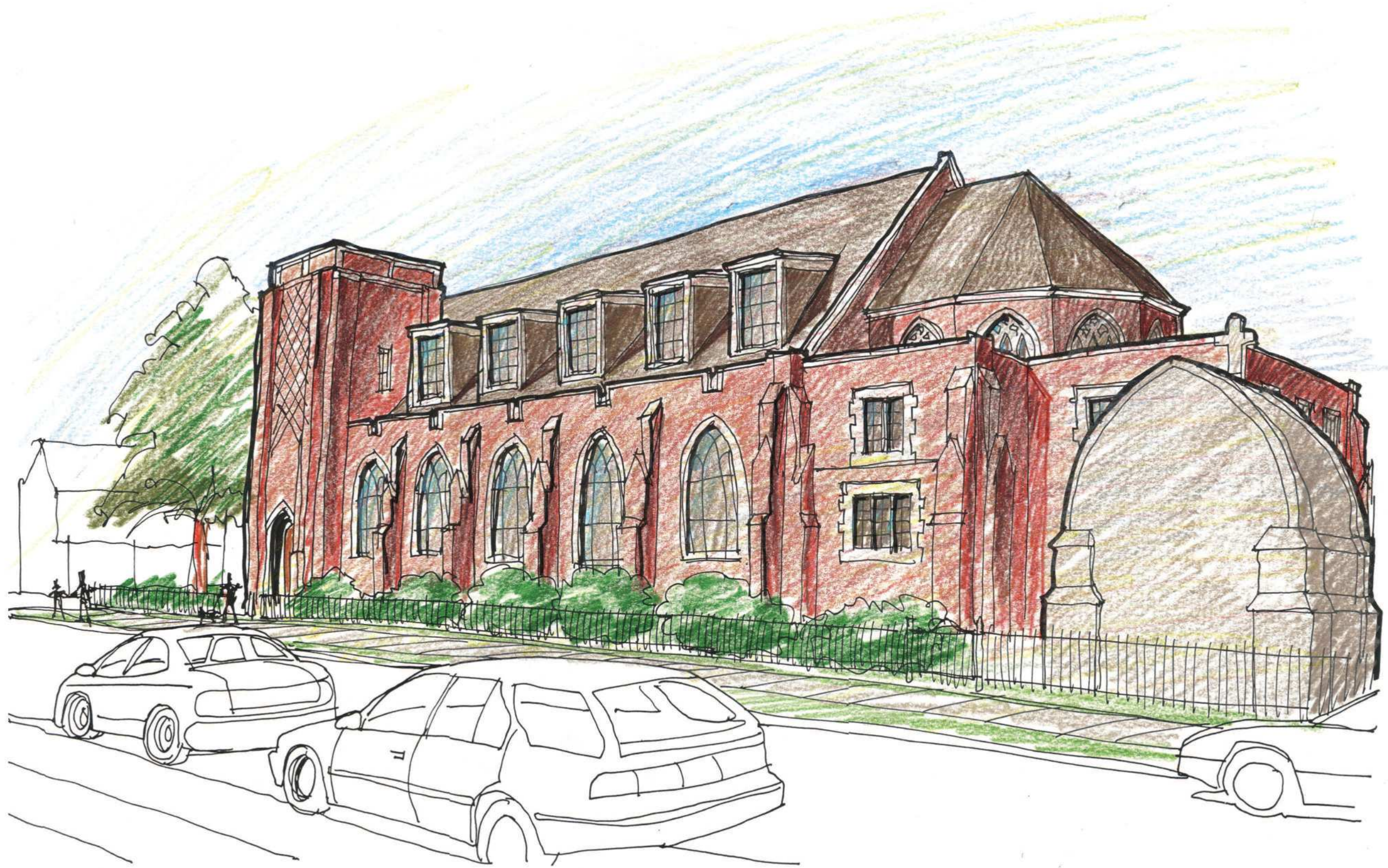
View of West 9 th Street Elevation with New Dormers
